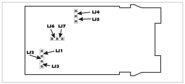
Figure 2-4 CPU PCB (Relay/SSR Drive/Solid State Output 1)
